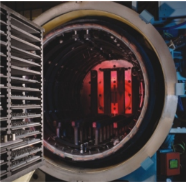
Precise control of Indo-MIM's vacuum sintering furnaces allows it to process a wide variety of materials.
